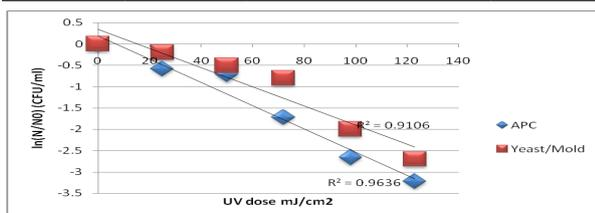
**Figure 1.** Dose response of bacteria and mold to UVC treatment
